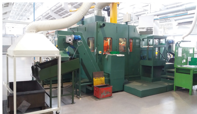
Fig. 1. Experimental stand for the screw forging process
