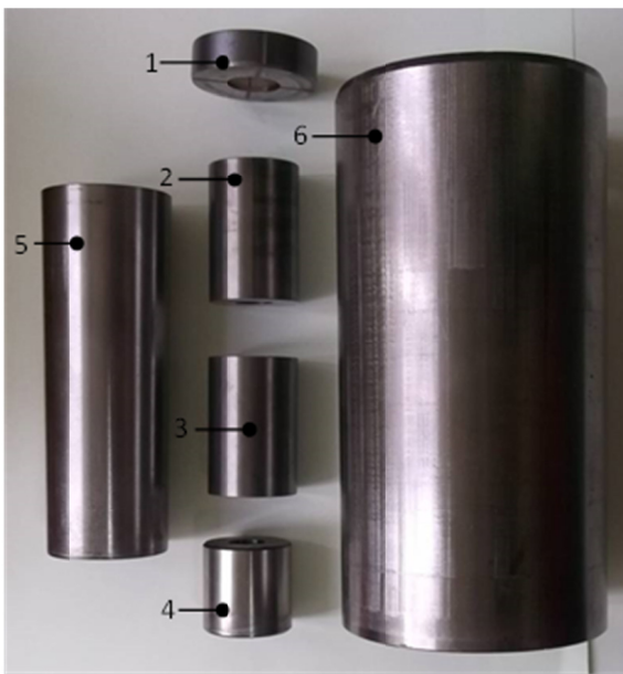
Fig. 3. The components of the tool die shaping operation for the fourth bolt: 1 – die, 2, 3, 4 – spacer sleeve, 5 – the centering tube blank, 6 – casing
