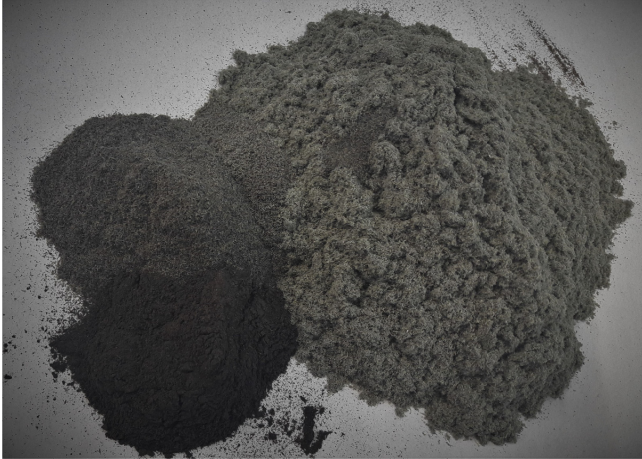
Fig. 3. Printed circuit boards after grinding in a mill
