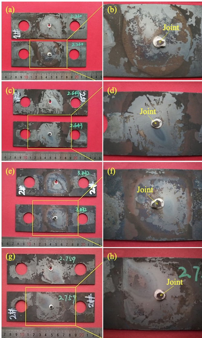
Fig. 7. Fracture morphology of the 7Mn welds after the cross-tension test: (a) and (b) are fractured sheets and joint after annealing at 800°C. (c) and (d) are fractured sheets and joint after annealing at 810°C. (e) and (f) are fractured sheets and joint after annealing at 820°C. (g) and (h) are fractured sheets and joint after annealing at 830°C
