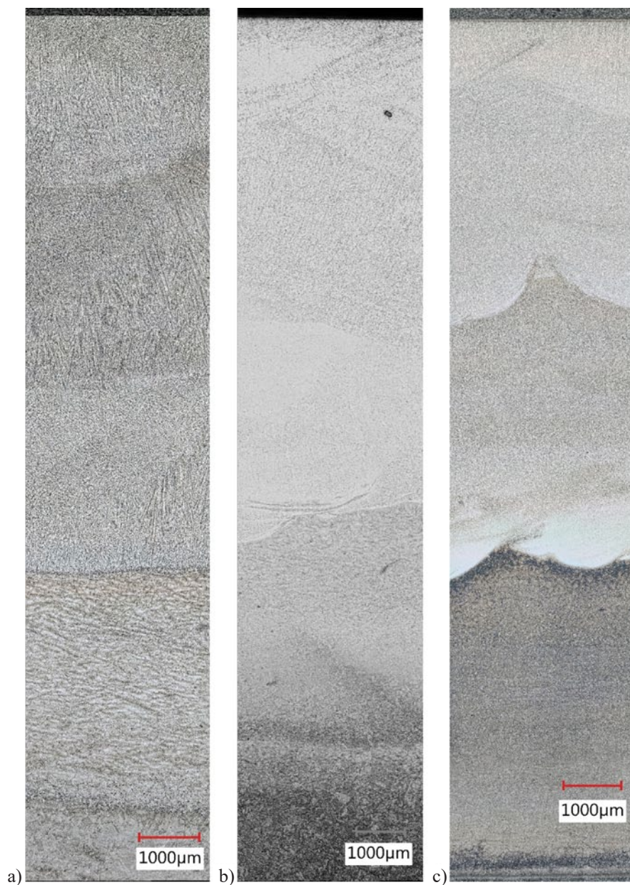
Fig. 15. Microstructure test results of samples made of a) DO*341, b) DO*04, c) DO*15
