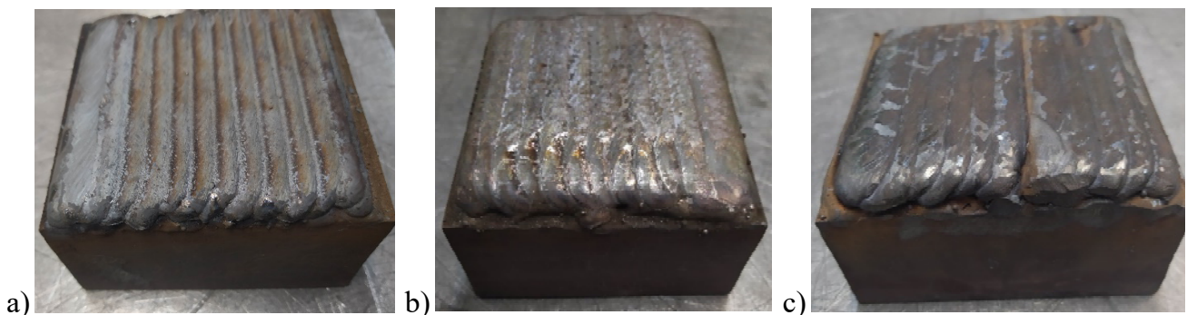
Fig. 14. Photographs of samples after the surfacing process: a) DO*341, b) DO*04, c) DO*15
