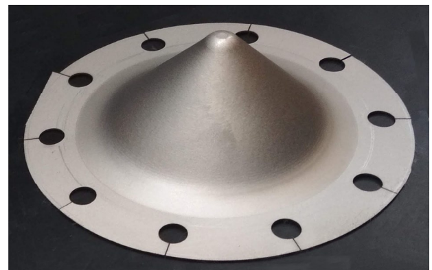
Fig. 3. One of the successfully obtained drawpieces
